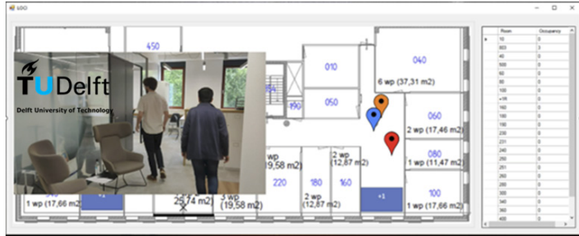
Figure 39: Location awareness using PIR/Thermopile (TU Delft)
