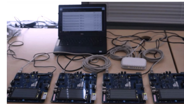
Figure 69: Demonstrator HistoTrust composed of decentralized electronic boards issuing attestations to an ethereum blockchain
