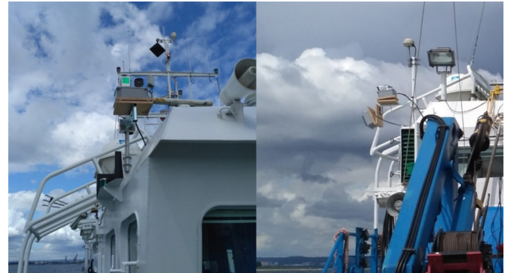
Figure 17: The Flexible Payload installed on m/v Tucana
