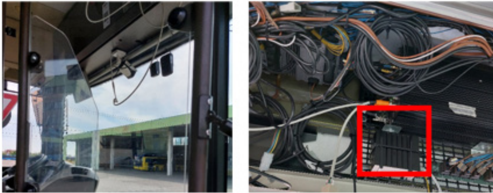
Figure 75: Potholes detection HW setup and sample frame for event detection
