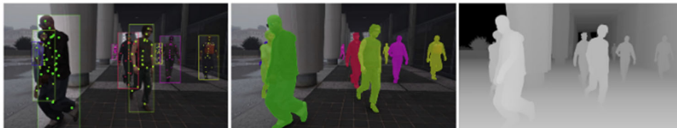
Figure 24 The visual representation of bounding box, segmentation, and depth map annotations in MOTSynth.
